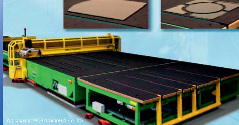
Cutting unit for laminated safety glass (VSG) from our partner company HEGLA with templates.
