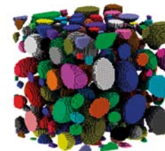
Microscopic representative volume cell of a casting slurry (only solid particles are illustrated).
