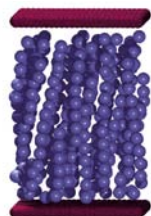
Simulation of the MRF in the shear field between two clutch discs.
