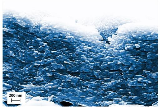
Fig. 1: REM image of the fracture edge of a  $Ti_2AIN$  coating with platelet-like shaped grains.
